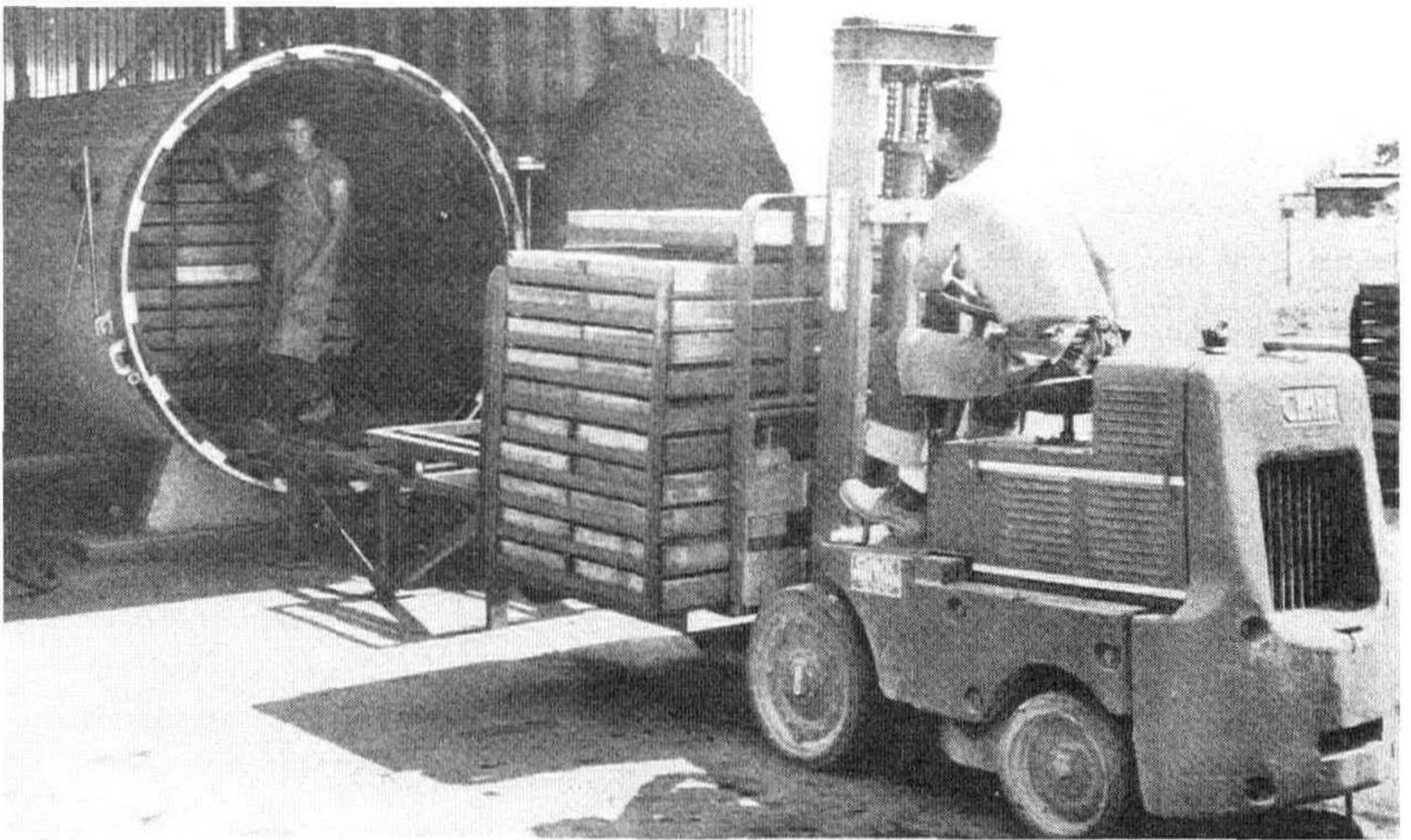
Figure 3. Cannery retort used for soil steaming in the mid-1940s. Free-flowing steam was used, and the soil held at 100°C for 30 minutes. Photo courtesy of American Plant Growers Inc., Carson, California.
