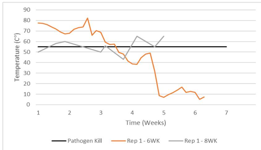
**Figure 2.** Temperature profiles of material in GORE® cells of the first composting cycle repetitions over time.
