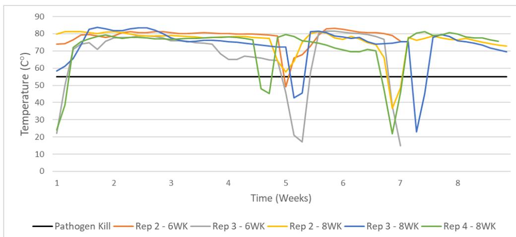
**Figure 4.** Temperature profiles of material in GORE® cells of composting cycle repetitions over time.
