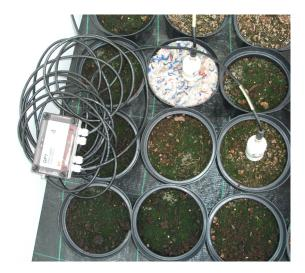
Fig. 4. Delta T moisture and temperature measurement equipment in place. Probes inserted in pot with pot cover and pot without pot cover.
