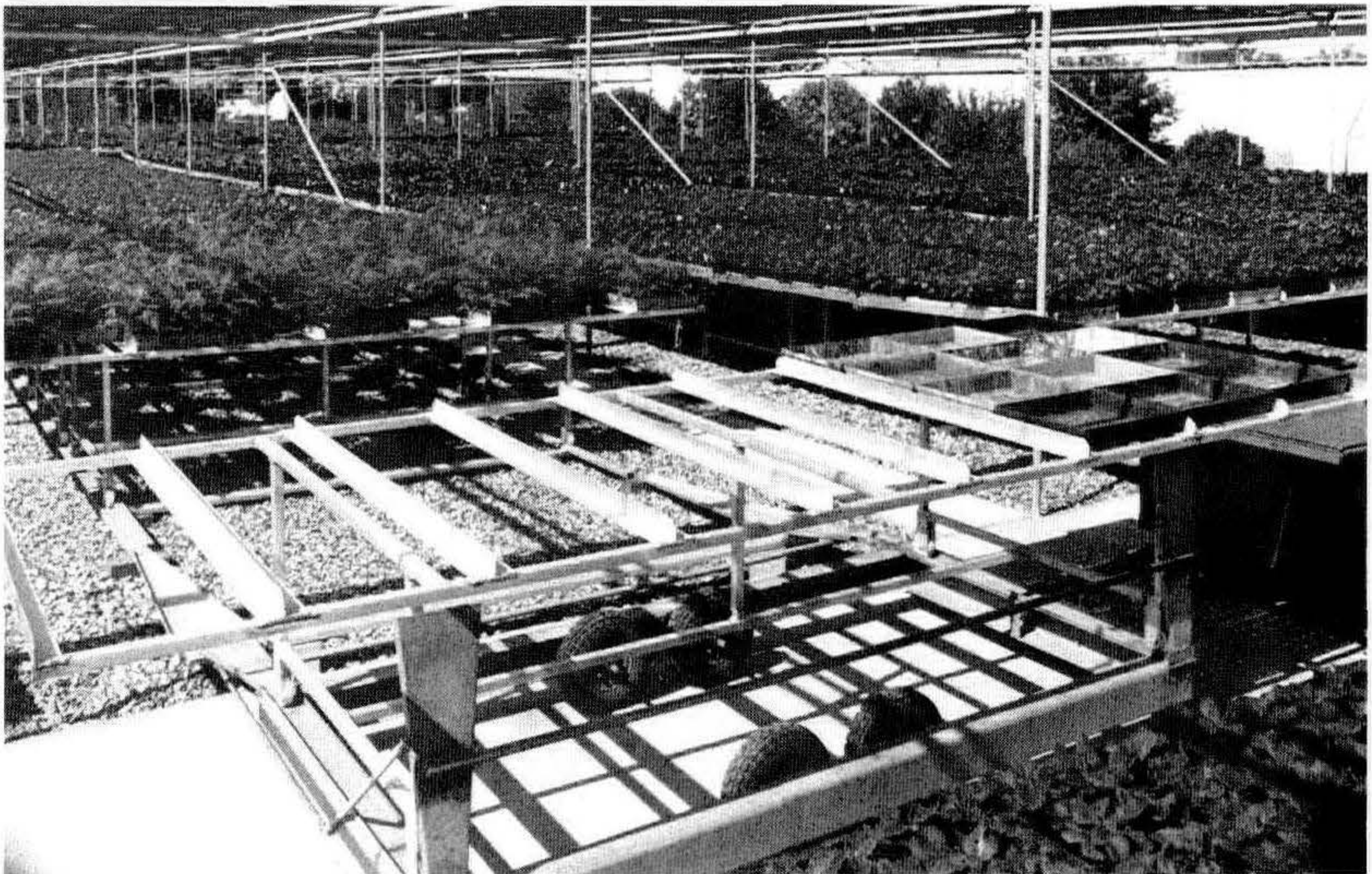
Figure 1. An aluminum frame which holds 36 plastic trays set in the rubber-tired trailer for moving. The frames are on four wheels, which run on two tracks. These frames are 500 mm high for good hygiene and for ease of handling. We used aluminum because of the rust problem with other metals and for the light weight. It cost a bit more, but it is worth it.
