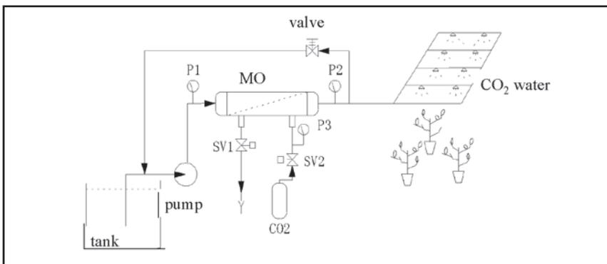
**Figure 1.** A view showing an example of plant-growing apparatus in the present paper. The apparatus is roughly made up of, from the upstream side, a water tank, a pressure pump, a hollow fiber membrane module MO, a CO<sub>2</sub> gas cylinder, a control valve SV2, and a relief valve. Operations of the entire apparatus are controlled by a control unit (not shown).
