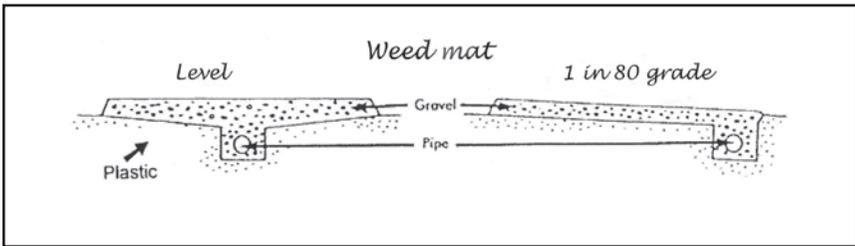
**Figure 2.** Floor construction in our production areas.
