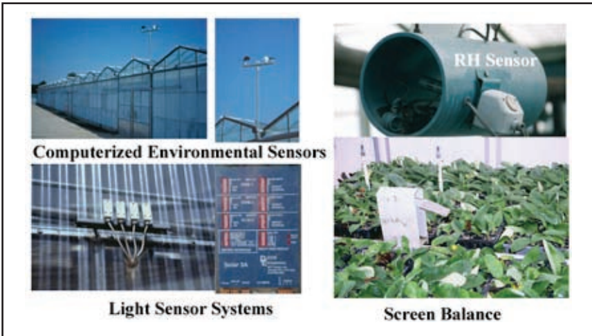
Figure 7. Dynamic mist control systems respond to changes in the environment affecting vapor pressure deficit. Evapotranspiration-based mist control systems (dynamic control) can respond to changes in air temperature, time interval between misting and calculated vapor pressure deficits between the leaf and surrounding air.
