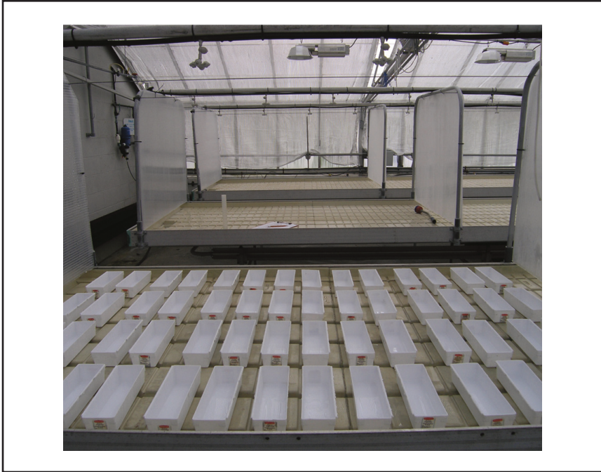
Figure 5. Collection trays set up to check for even mist nozzle coverage.
